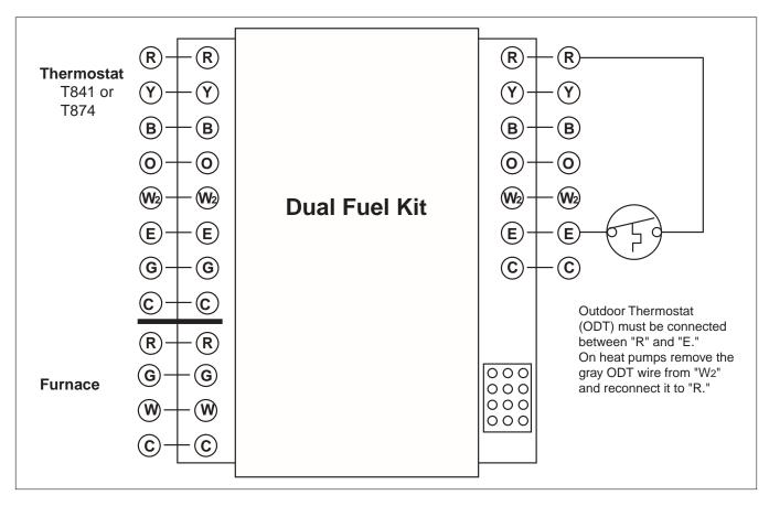
Figure 1. Dual Fuel Kit Terminal Location and System wiring Diagram
