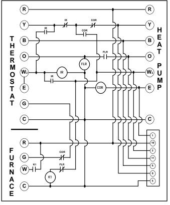
Figure 3. Dual Fuel Kit Electrical Schematic
