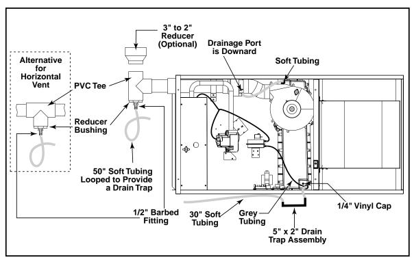
Figure 4. 90+ Upflow Converted for Horizontal Installation (Horizontal Left)
