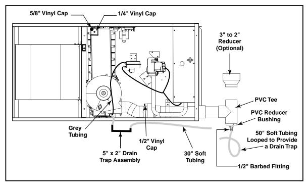
Figure 3. 90+ Upflow Converted for Horizontal Installation (Horizontal Right)
