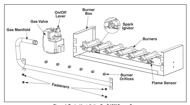
Figure 1. Typical Installation For R4GM Burner Box
