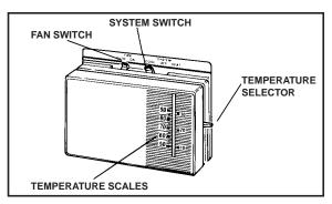
Figure 1. Typical Thermostat
