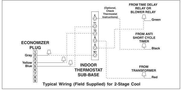
Figure 8. Typical Thermostat Connection
