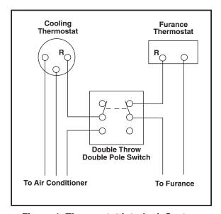
Figure 1. Thermostat Interlock System
