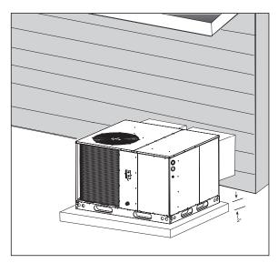
Figure 5. Ground Level Installation
