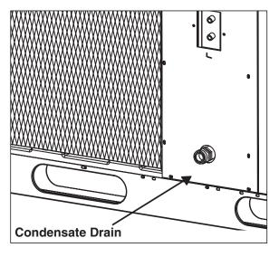
Figure 4. Condensate Drain
