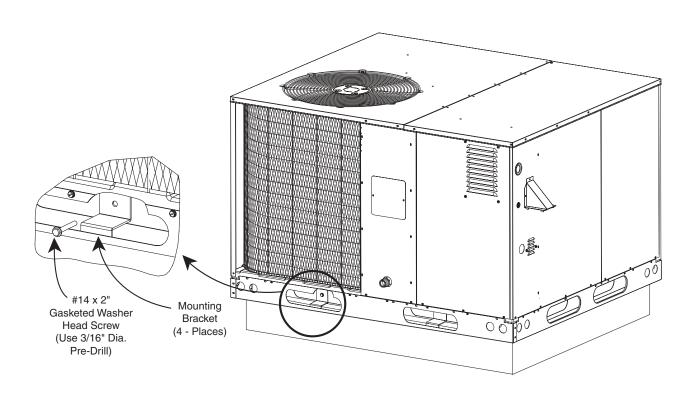
Mounting system depicted is suitable for mounting to a standard roof curb at a height above ground up to 60 feet. Suitable mounting up to 500 feet above ground may be accomplished by using a 14 ga. curb and 2 clips in each mounting pocket.
