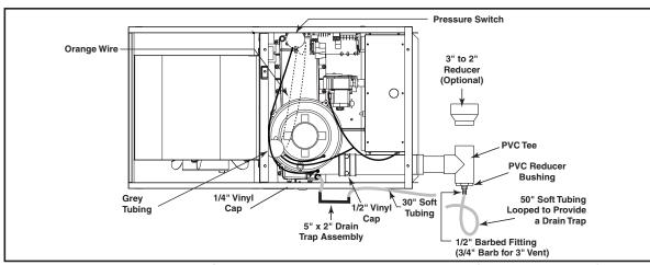
Figure 3. 90+ Upflow Converted for Horizontal Installation (Horizontal Right)
