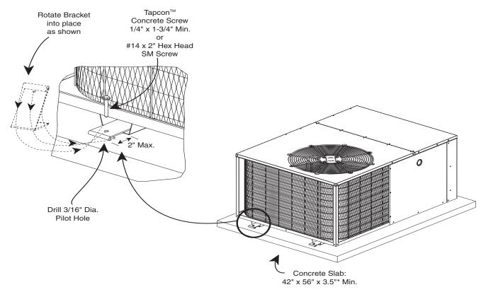
\*Slab may be less than 3.5" but not less than 2" if allowed by all applicable codes
