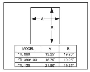
Figure 5. Opening for Concrete Slab
