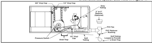
Figure 3. 90+ Upflow Converted for Horizontal Installation (Horizontal Right)
