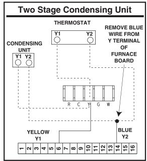
Figure 27. Two Stage Condensing Unit
