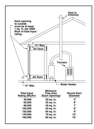
Figure 15. Equipment in a Confined Space with all Combustion Air Drawn from the Outside through Horizontal Ducts
