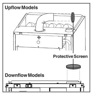
Figure 10. Protective Screen for One Pipe Installations
