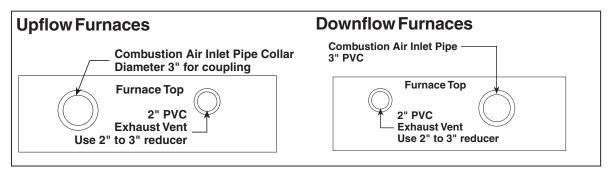
Figure 18. Furnace Pipe Adaptions
