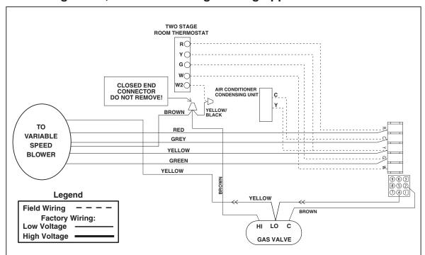
Figure 26a. Two Stage Configuration
