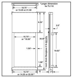
Figure 9. Downflow Sub-Base Dimensions
