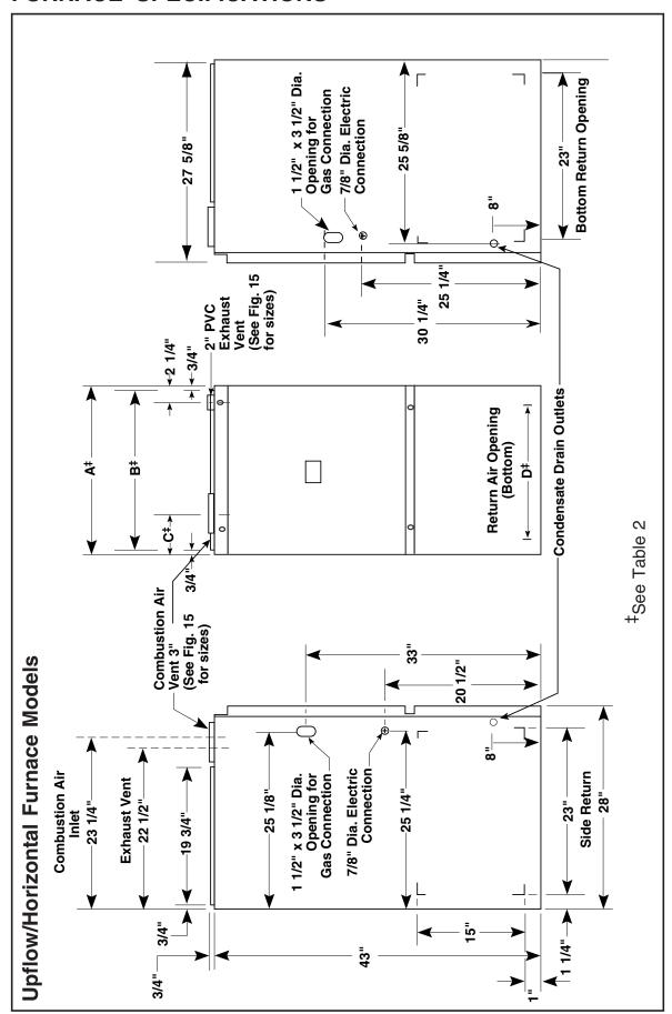
Figure 1. Upflow/Horizontal Unit Dimensions
