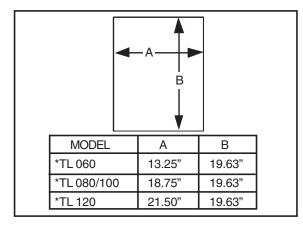
Figure 7. Opening in Wood Floor
