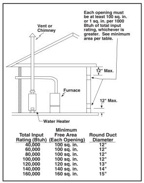
Figure 11. Equipment in a Confined Space with all Combustion Air drawn from Inside
