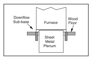
Figure 8. Furnace on a Wood Floor
