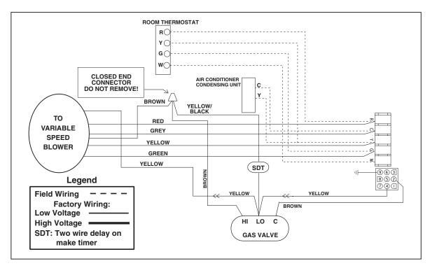
Figure 26e. Timed Two Stage Configuration
