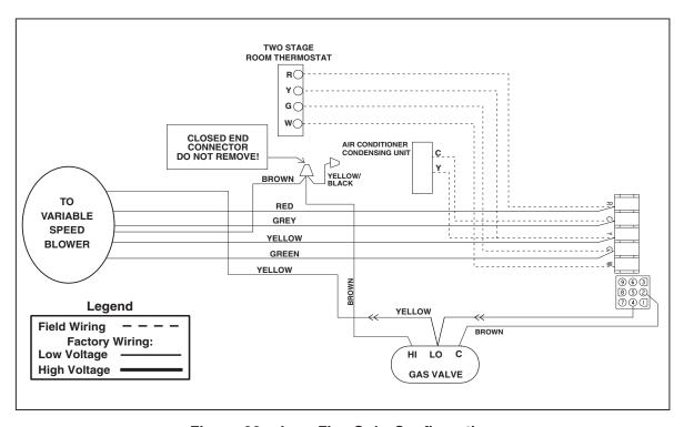
Figure 26c. Low Fire Only Configuration
