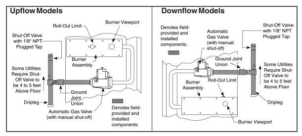
Figure 24a. Typical Gas Service Connection
