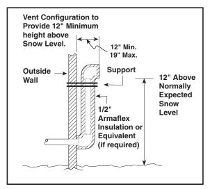
Figure 20. Alternate Horizontal Vent Installation
