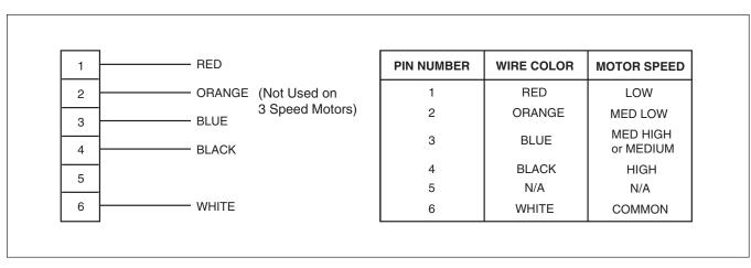
Figure 8. Indoor Blower Motor Leads.
