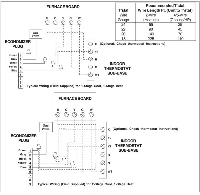
Figure 9. Typical Thermostat Connections.
