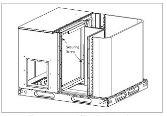
Figure 3a. Internal Filter Rack Location
