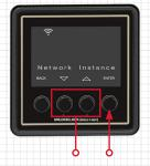
Using up or down arrows, navigate to "Network Instance"
