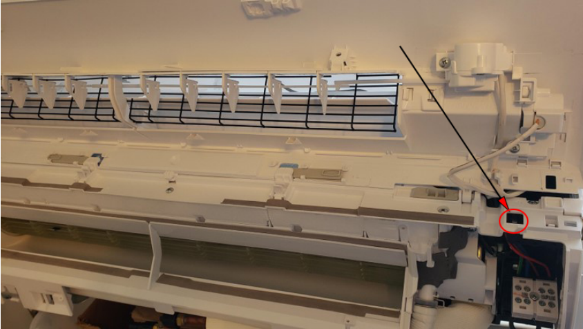
Fig. 510 (Door Micro Switch)
