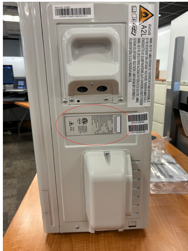
Figure 102 (Indoor Unit Model Nameplate location)
