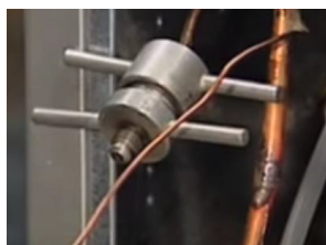
Process tube adapter kit
