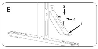
Step 1: Align Angle Bracket to leg and upright
