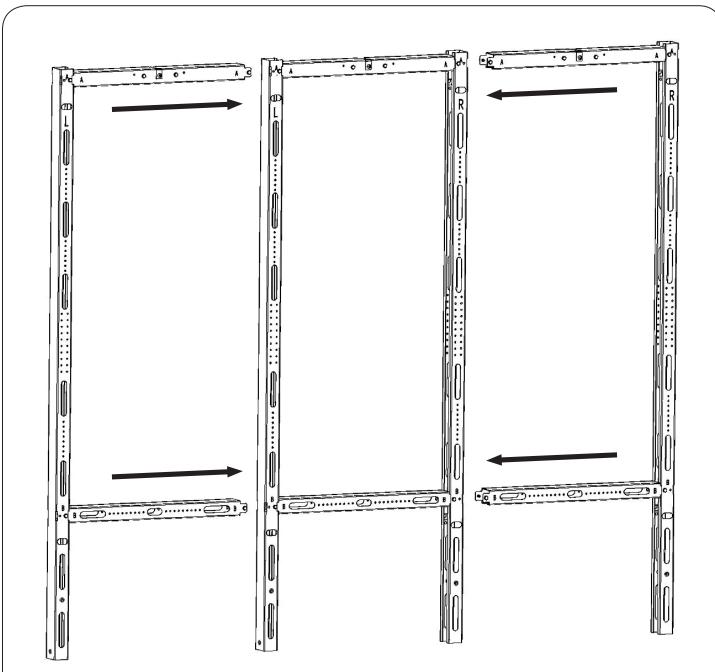
Units may be expanded by purchasing additional EZ-Rack™ Kits and adding to the left or right side by repeating steps A, B, and C. In this case not all parts will be used. For additional free standing base or wall mounts, repeat steps D, E, and F from corresponding page.
