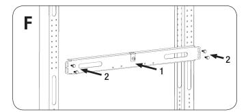
Step 1: Place Cross Bar against the uprights according to the size of the heater you are installing
