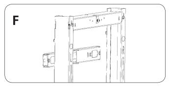
Step 1: Hook the frame onto the leg on the wall and secure using ¼-20 fasteners
