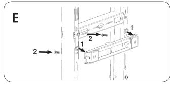
Step 1: Hook the second leg into the back of the frame below B
