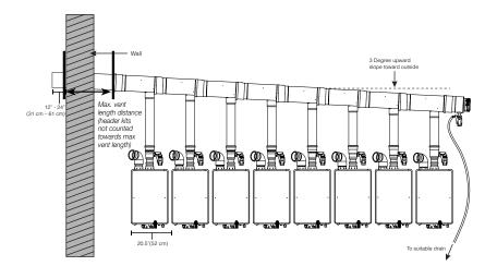
These kits contain only minimum required vent parts to create a common venting trunk line and a connection from the trunk line to water heaters. Vent parts included in these kits **DO NOT** count for equivalent vent length except a 87 degree elbow for the air intake included in a room air kit. Additional vent parts will be required to complete the common venting system. Refer to "Parts List" of this installation instructions for additional information.
