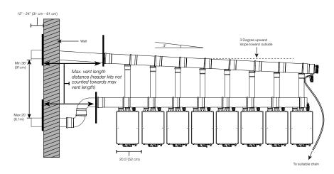
RHEEM **TRUNK NUMBER OF UNITS PART NUMBER** DIAMETER SP20906A 2 6" 3 SP20906B SP20906C 4 SP20908A 2 SP20908B 3 SP20908C 4 SP20908D 5 8" SP20908E 6 SP20908F 7 SP20908G 8 SP20910A 2 SP20910B 3 SP20910C 4 SP20910D 5 SP20910E 10" 6 SP20910F 7 SP20910G 8 SP20910H 9 SP20910J 10
